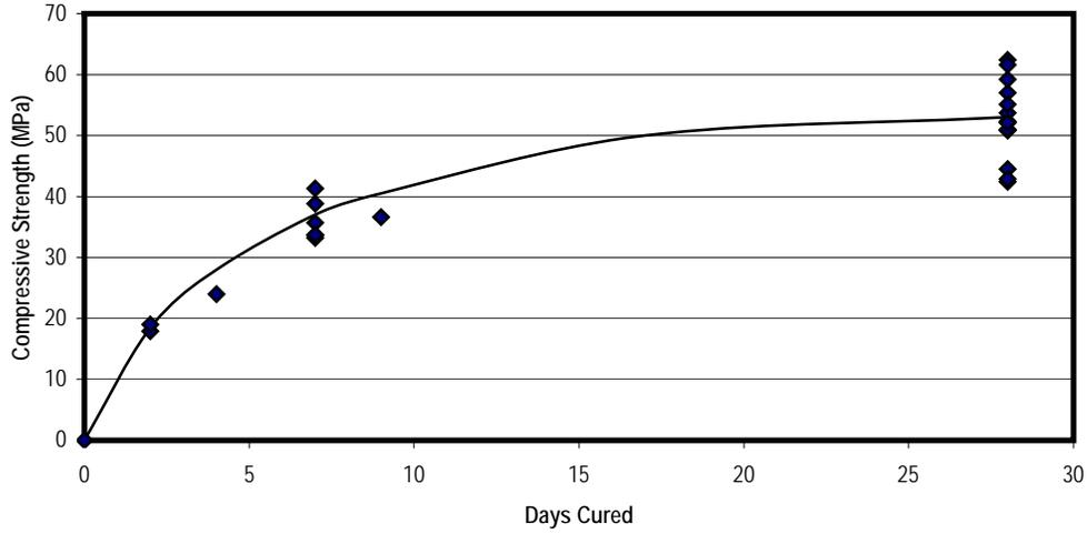
**Table 11: Compressive strength test data for horizontally applied dry process shotcrete
