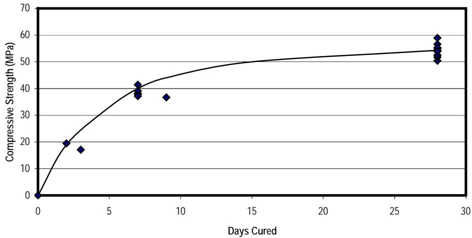
**Table 12: Comparison of compressive strength test data for horizontally and vertically applied dry process shotcrete, Spray-Con DS ST
